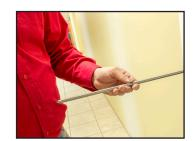
Do not reverse the drill while the multi-sectioned bit is in the raceway. This could unscrew sections of the drill bit.
