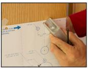
2. Hand tighten the drill bushing screw on the other side of the door. Let the tool rest on the edge of the door as shown.
