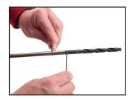
If you are using the multi-piece drill bit, start out with 2 sections of the bit joined together and add sections as the raceway depth increases.
